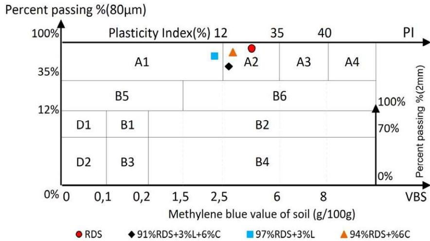
Fig. 8. Classification of the RDS according to the soil classification table of the NF P11-300 standard (Association Française de Normalisation, 1992a) (fraction 0/50 mm)
