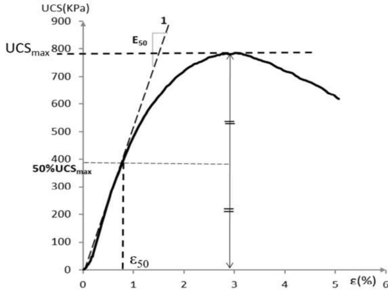
Fig. 11. Secant modulus  $E_{50}$  versus strain ( $\epsilon$ )
