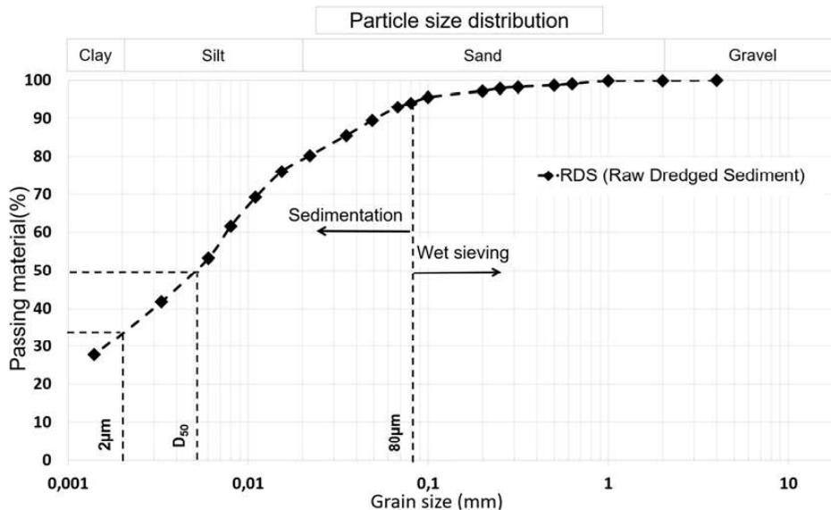
Fig. 2. Particle size distribution of the RDS
