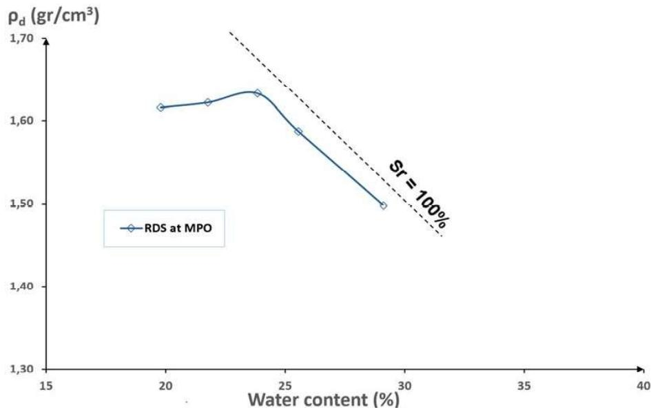
Fig. 4. Compaction tests at MPO for the RDS
