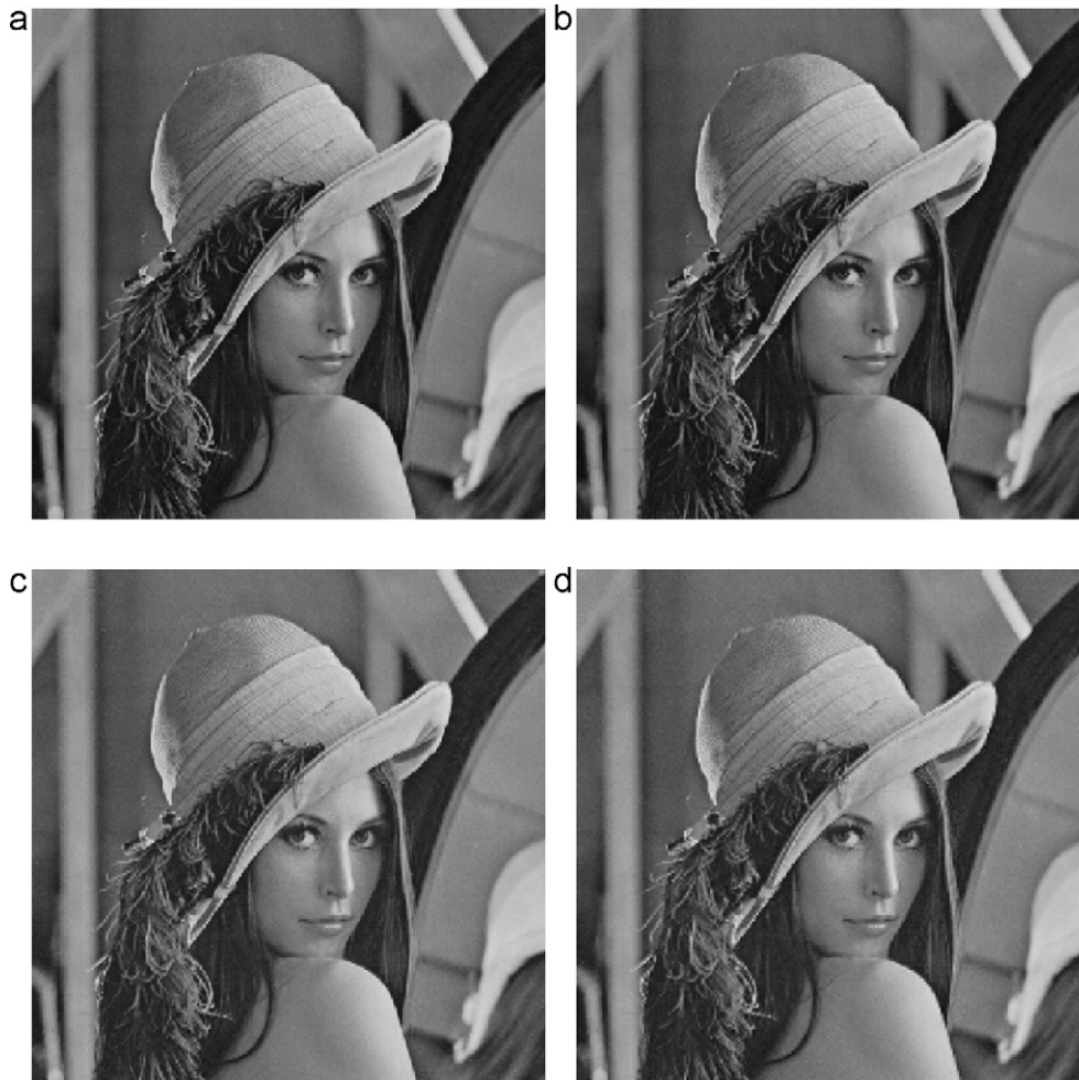
Fig. 6. Lena image reconstruction results for MDTC.DWT/UQ at 2.0 bits/sample (a) reconstructed image from the 4 received packets (PSNR=46.88 dB); (b) reconstructed image from 3 received packets (PSNR=43.12 dB); (c) reconstructed image from 2 received packets (PSNR=36.12 dB); (d) reconstructed image from 1 received packet (PSNR=32.67 dB).
