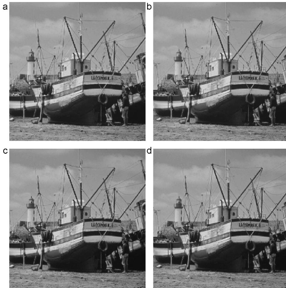
Fig. 11. Boat image reconstruction results for MDTC_DWT/SUQ at 2.0 bits/sample (a) reconstructed image from the 4 received packets (PSNR = 39.35 dB); (b) reconstructed image from 3 received packets (PSNR = 38.84 dB); (c) reconstructed image from 2 received packets (PSNR = 35.08 dB); (d) reconstructed image from 1 received packet (PSNR = 30.44 dB).
