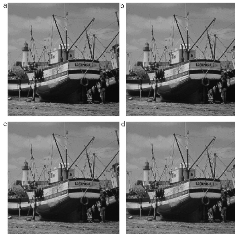
Fig. 10. Boat image reconstruction results for MDTC_DWT/UQ at 2.0 bits/sample (a) reconstructed image from the 4 received packets (PSNR = 39.67 dB); (b) reconstructed image from 3 received packets (PSNR = 38.92 dB); (c) reconstructed image from 2 received packets (PSNR = 32.88 dB); (d) reconstructed image from 1 received packet (PSNR = 28.41 dB).
