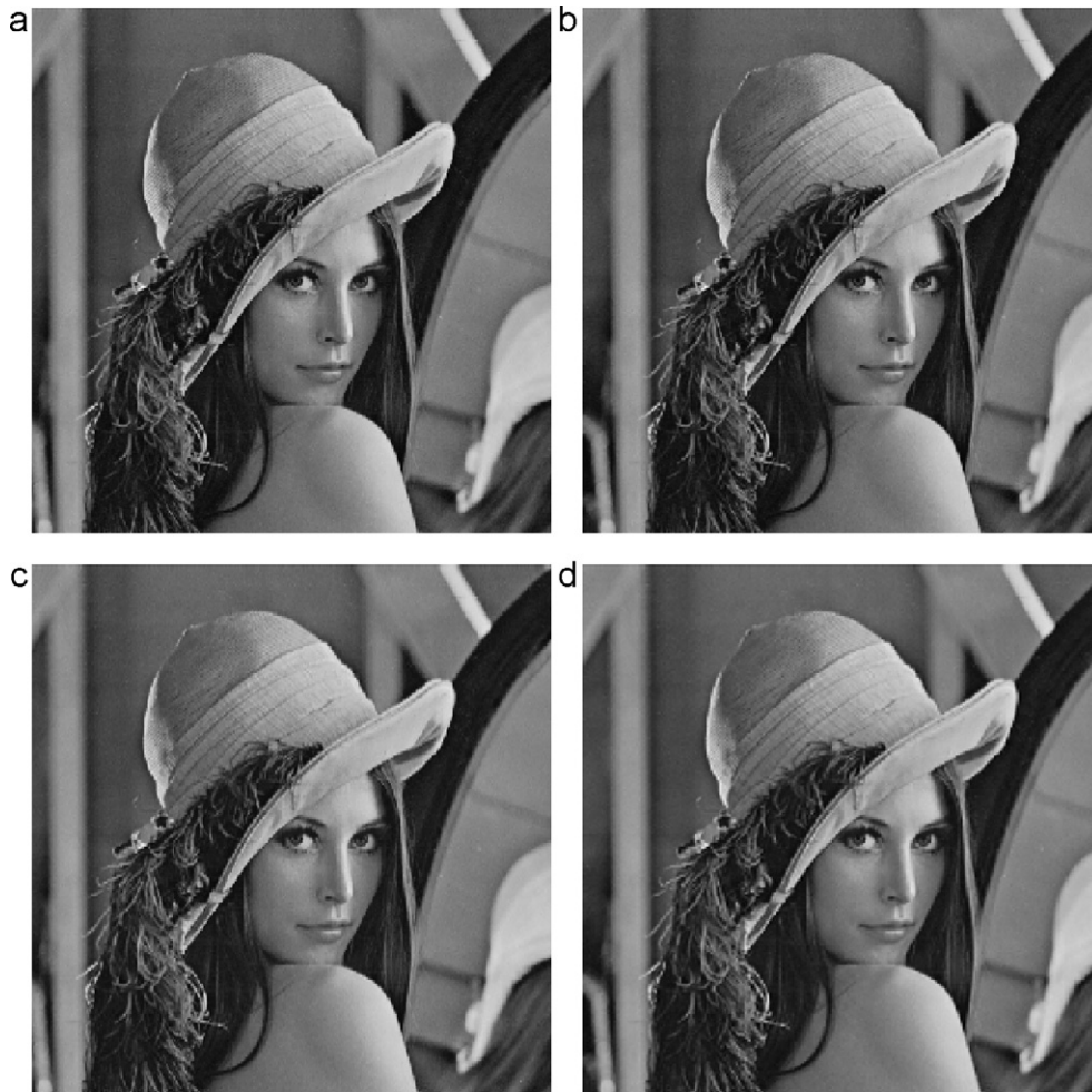
Fig. 7. Lena image reconstruction results for MDTC.DWT/SUQ at 2.0 bits/sample (a) reconstructed image from the 4 received packets (PSNR=43.96 dB); (b) reconstructed image from 3 received packets (PSNR=41.97 dB); (c) reconstructed image from 2 received packets (PSNR=38.09 dB); (d) reconstructed image from 1 received packet (PSNR=34.44 dB).
