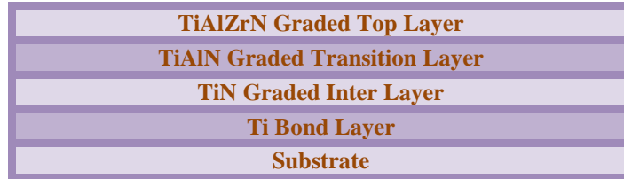
Figure 1. Design concept of the graded composite of TiAlZrN coating
