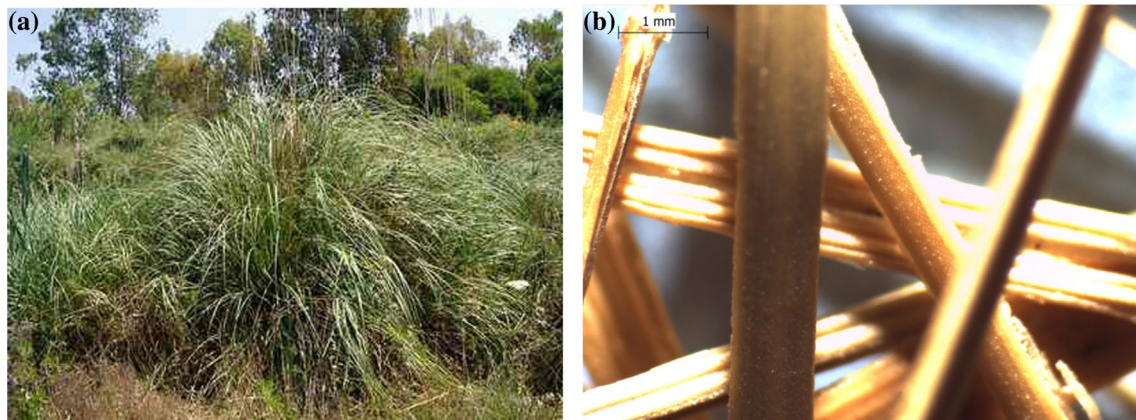
Fig. 3 The DISS fibre ( Ampelodesma mauritanica ); a the natural state, b the raw state
