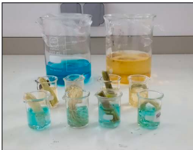
Fig. 5. The filtration process of the two organic dye solutions.
