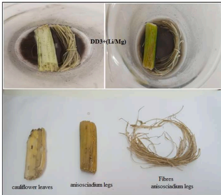
Fig. 4. The new shape of the samples after deposition of (Li/Mg)+DD3 using cauliflower leaves and anisosciadium legs and their fibers.
