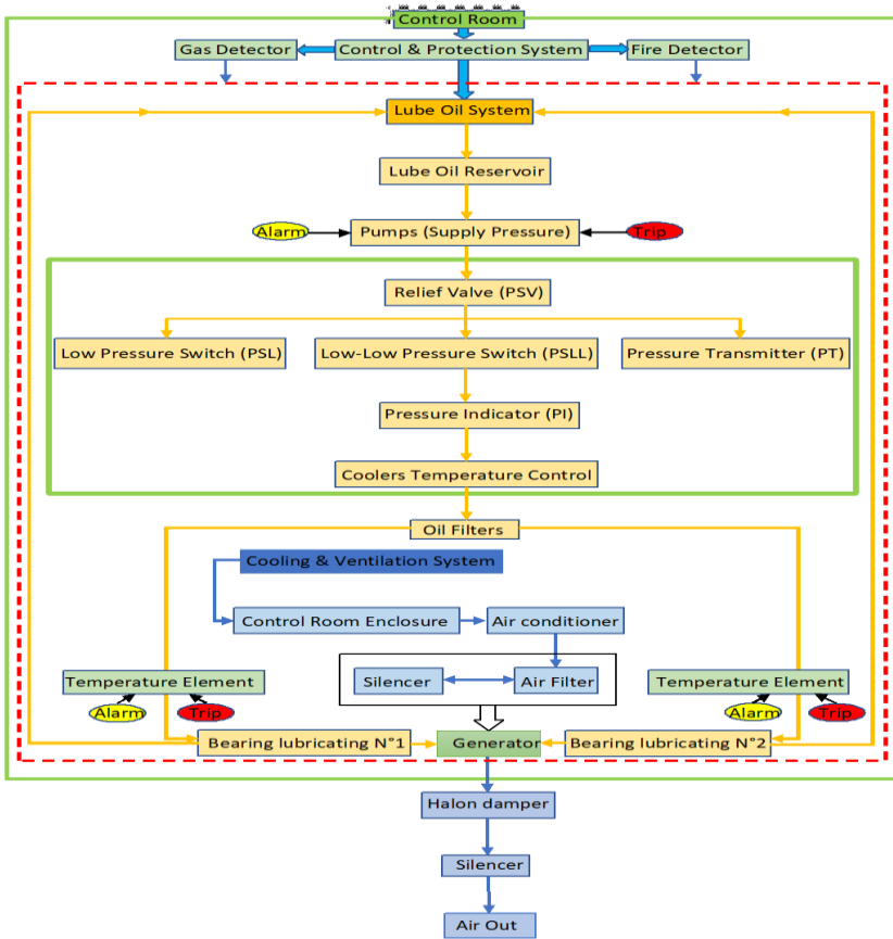
Figure 1: Schematic diagram of a generator protection system.
